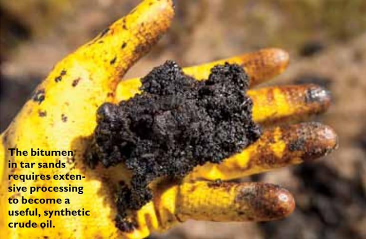
**The bitumen in tar sands requires extensive processing to become a useful, synthetic crude oil.**
