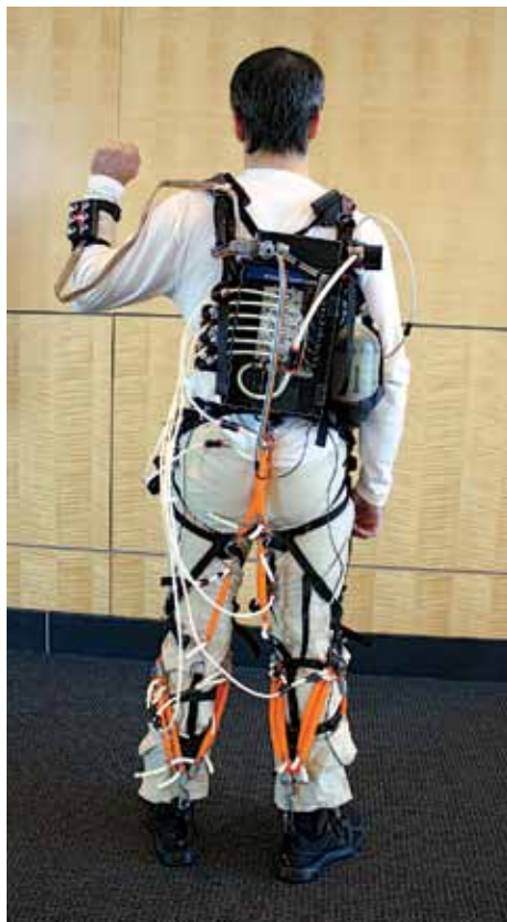
Conor Walsh’s lab is designing a robotic “exosuit” to aid human movement; soft and lightweight, it can be worn under clothes.
